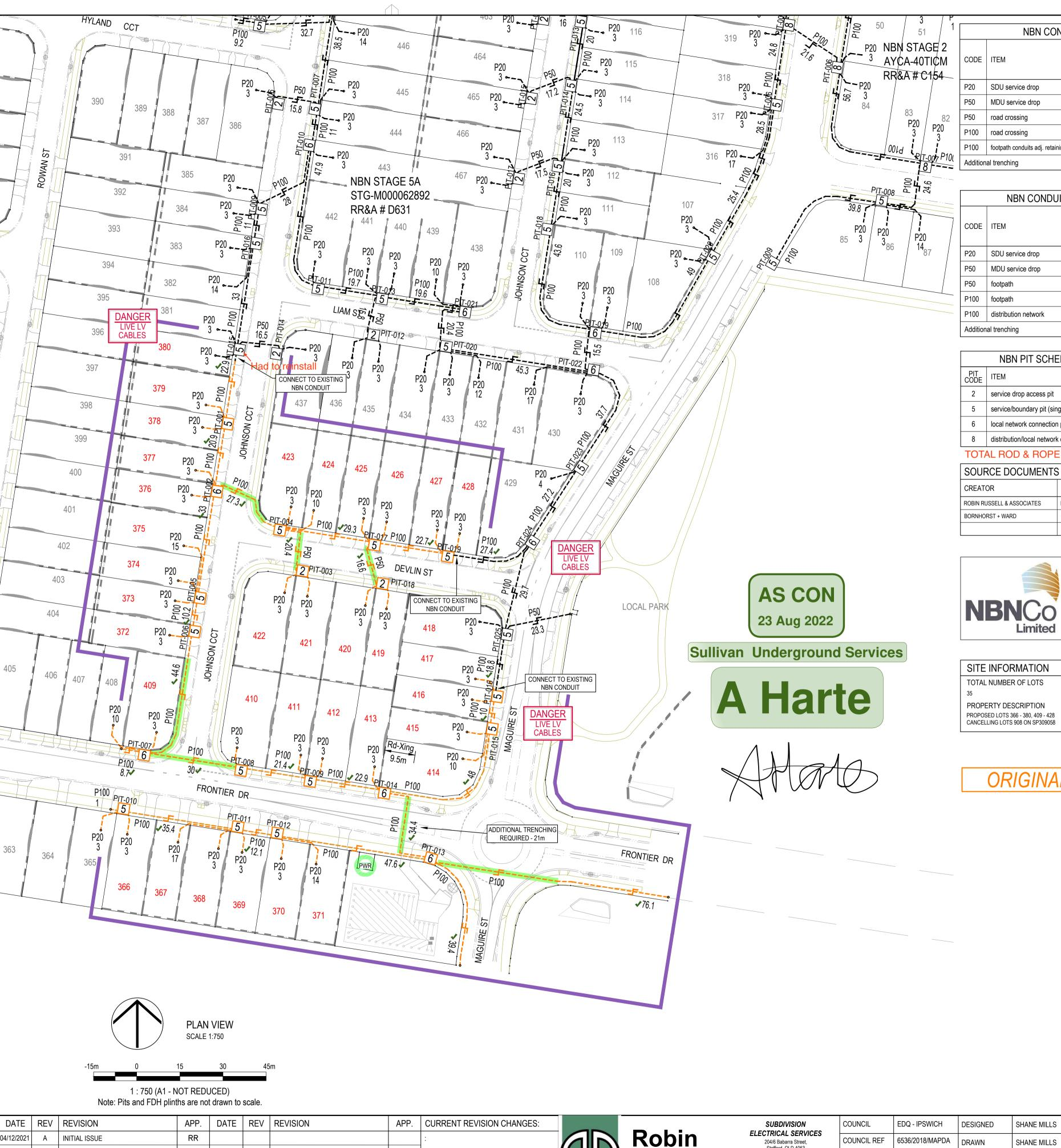
NBN CONDUIT SCHEDULE - CIVIL CONTRACTOR Refer: AS/NZS 1477:2006 - Table 4.2(A) QUANTITY CODE | ITEM MEAN MEAN THICKNESS OUTSIDE DIA. INSIDE DIA P20 SDU service drop PN12 27mm 24mm P50 MDU service drop PN12 60mm 54mm PN12 31 54mm road crossing 60mm PN9 102 P100 road crossing 114mm 104mm P100 | footpath conduits adj. retaining walls 104mm 42 PN9 114mm 21 Additional trenching
